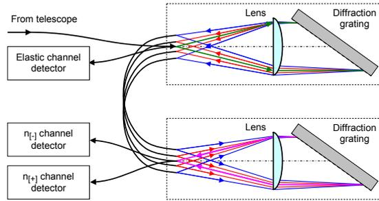
Fig. 4: Example of a diffraction-grating polychromator. Footnotes [+ ] and [- ] indicate two channels with positive and negative temperature sensitivity.
