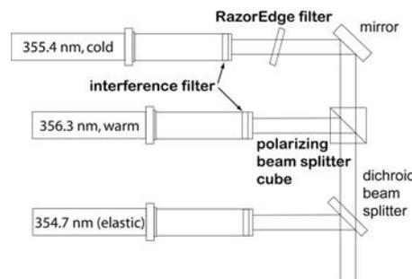
Fig. 3: Part of the MARTHA receiver setup showing the rotational Raman channels and the elastic-backscatter channel for the emission wavelength of 354.7 nm.
