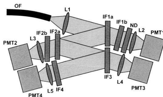
Fig. 2: Sequential interference filter setup for the measurement of rotational Raman signals (with PMT2 and PMT3), elastic backscattering (with PMT1) and  $N_2$  vibration-rotation Raman scattering (with PMT4). OF, optical fiber; L1–L5, lenses; IF1a–IF4, interference filters; ND, neutral density attenuator; PMT1–PMT4, photomultiplier tubes. Figure taken from Behrendt and Reichardt [2000].
