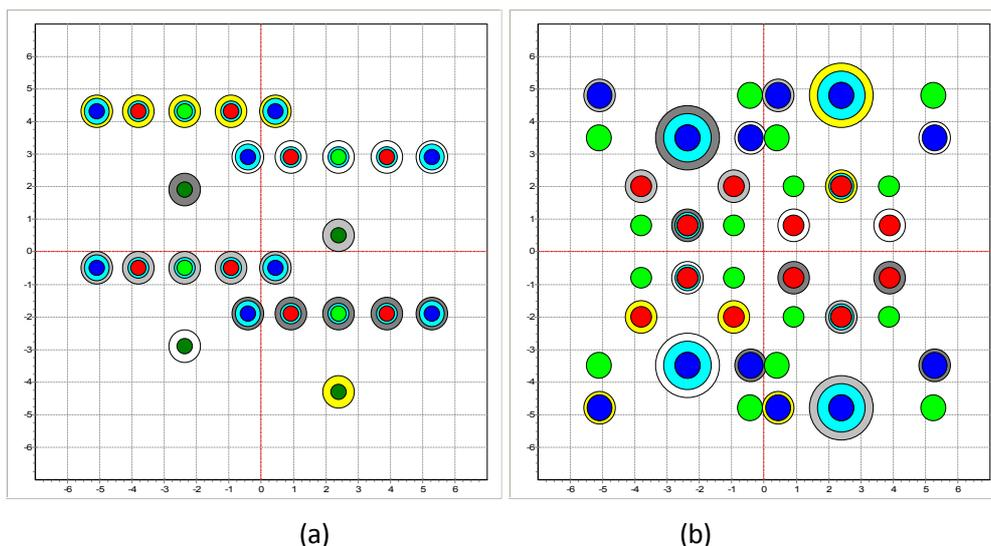
Fig.6. Fiber assembly of first (a) and second (b) polychromator chamber for the four-telescope configuration of the MPI Raman lidar. Different colors of fiber cladding (white, light gray, dark gray, yellow) mark four different input channels.
