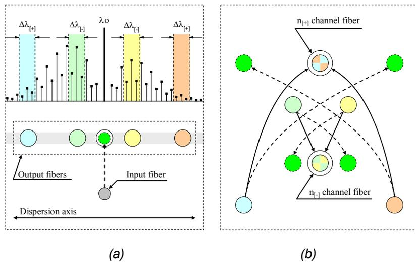
Fig. 5: Fiber arrangement in the lens focal plane of the first (a) and second (b) chamber of the polychromator. Dashed and solid arrows indicate the position of the fiber image for elastic and inelastic light, respectively. The spatial distribution of PRRS of nitrogen in diffracted light is schematically shown in panel (a).
