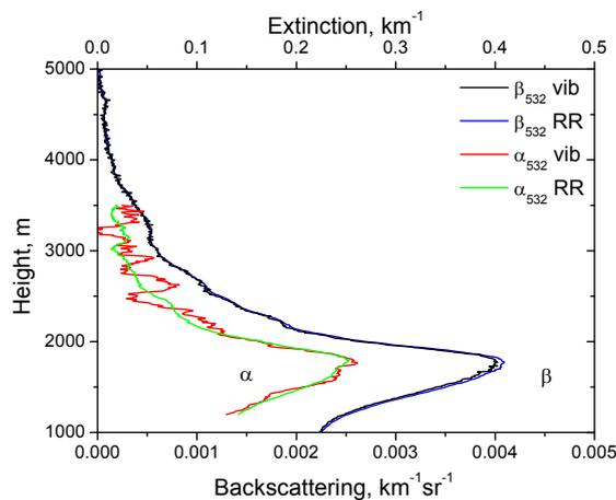
Figure 2: Extinction and backscatter coefficients at 532 nm computed from nitrogen vibrational Raman (vib) and from PRRS signal (RR).
