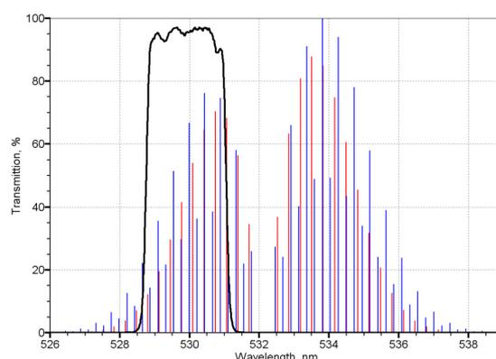
Figure 1: PRRS of nitrogen (blue) and oxygen (red) for  $T = 300$  K. The black line shows the transmittance of the interference filter used in the experiment. In this case, the laser line is at 532.12 nm (Veselovskii et al., 2015b).
