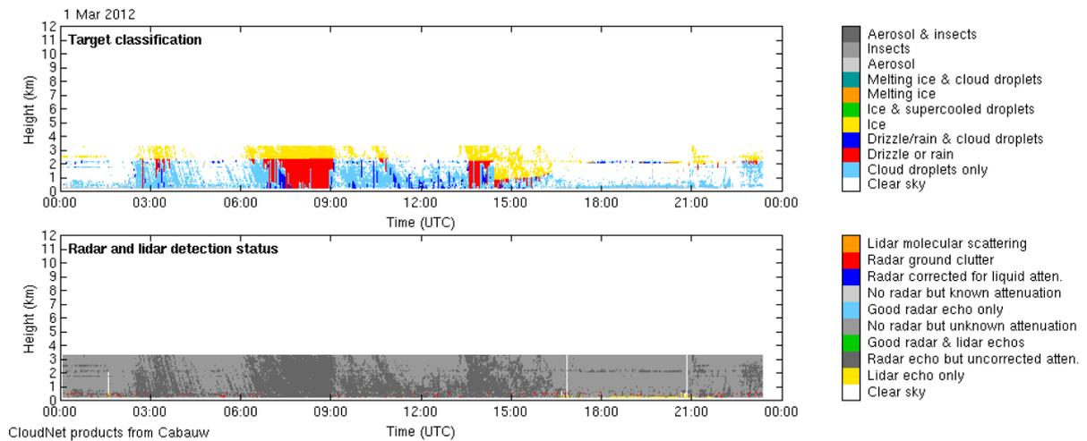
Figure 1. An example of a Cloudnet Target Classification and Radar and lidar detection status products.
