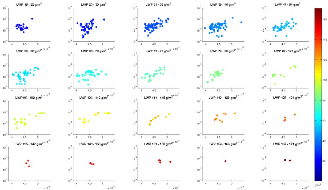
Figure 3. An example of a scatter plots comparing Lidar Attenuated Backscatter Coefficient (x axis) and Radar Reflectivity Factor (y axis). Data is divided into bins of LWP. *Source: Sarna Karolina, Russchenberg, H.W.J., "Framework for monitoring aerosol-cloud interactions in liquid water clouds" 4th ACTRIS General Meeting, June 10-13 2014, Clermont-Ferrand, France.*
