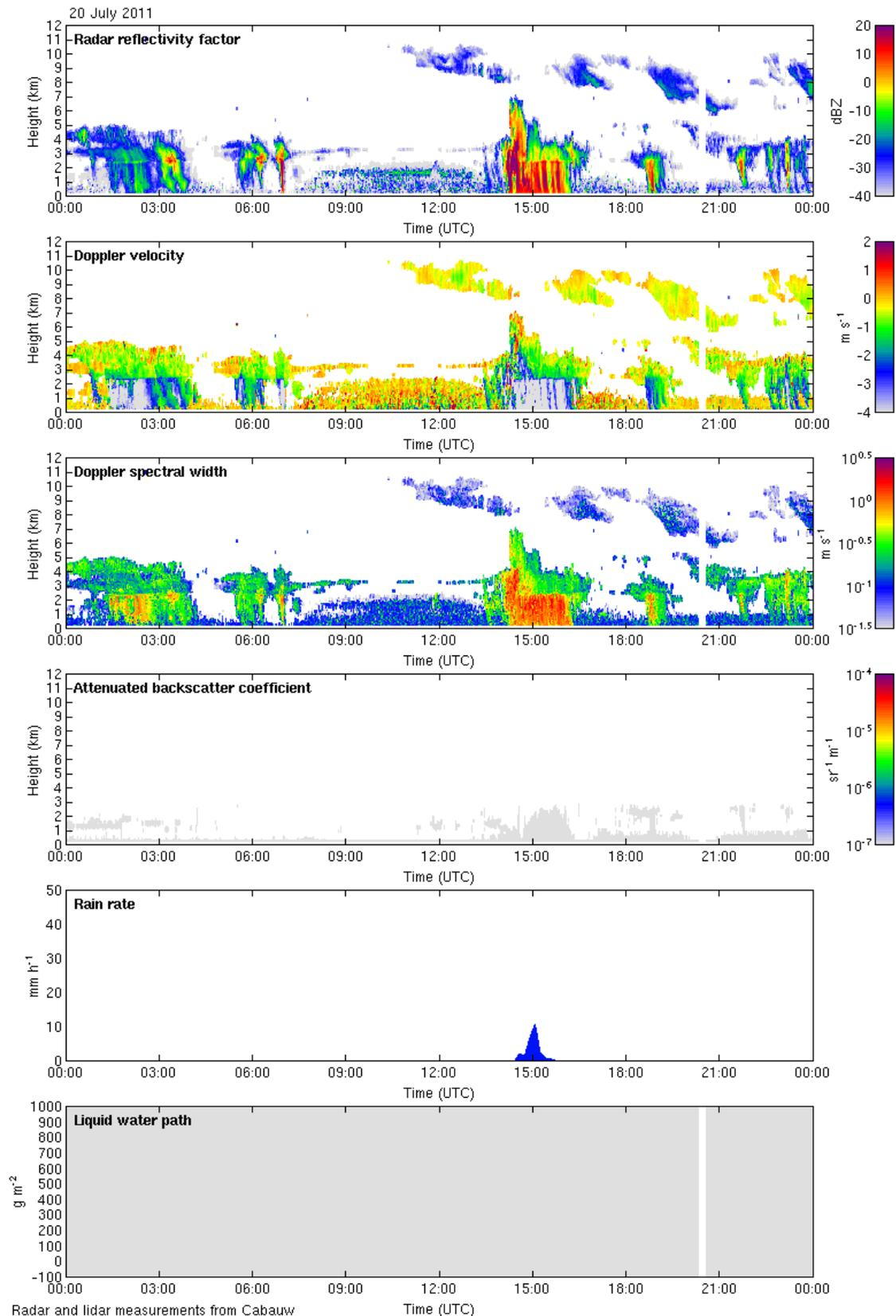
Figure 2. An example of Cloudnet Processed radar and lidar measurements (Level 1c) product. Source: [http://www.cloud-net.org/radar/cloudnet/quicklooks/cabauw\\_measurements.html](http://www.cloud-net.org/radar/cloudnet/quicklooks/cabauw_measurements.html)
