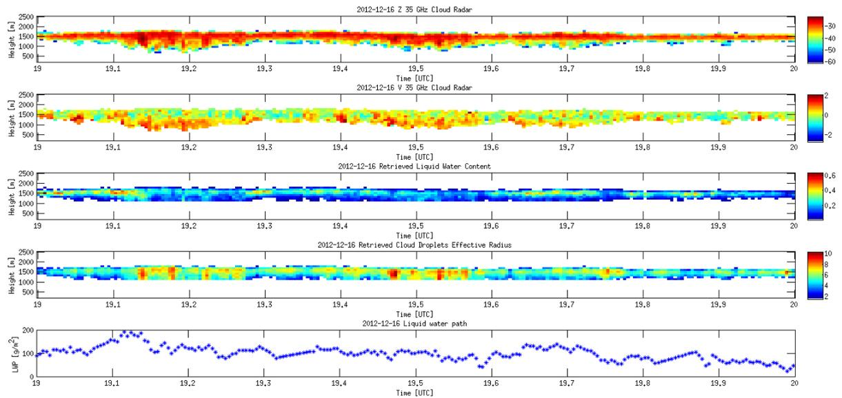
Figure 5. An example of the output from the Liquid Water Cloud Properties Retrieval.
