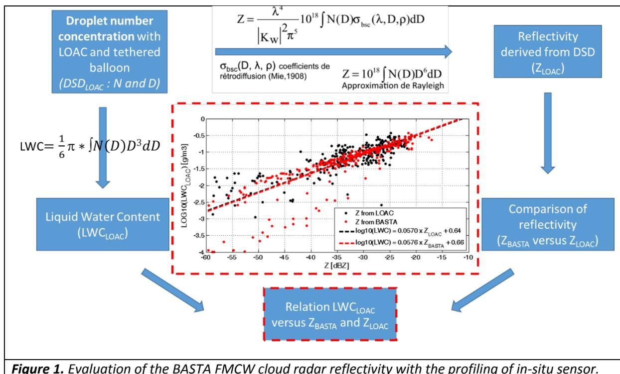
**Figure 1.** Evaluation of the BASTA FMCW cloud radar reflectivity with the profiling of in-situ sensor.
