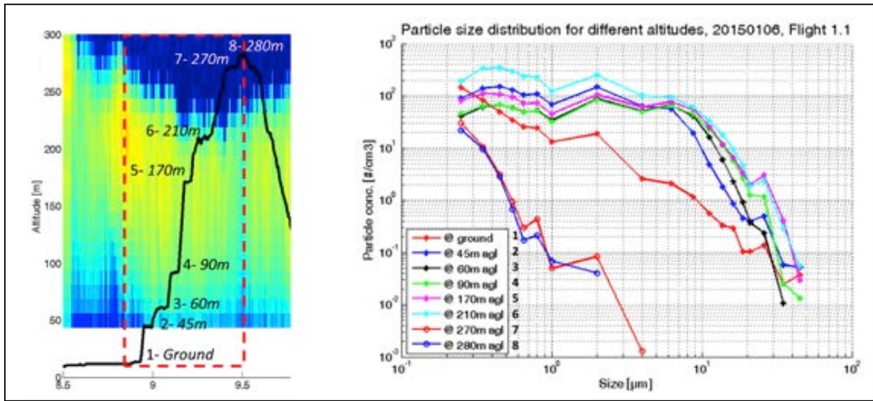
**Figure 7a.** Tethered balloon flight equipped with the LOAC sensor and associated droplet size distribution along the vertical. Left: radar reflectivity profile during 1 hour, and altitude of the in-situ sensors. Right: size distributions obtained at the different altitudes.
