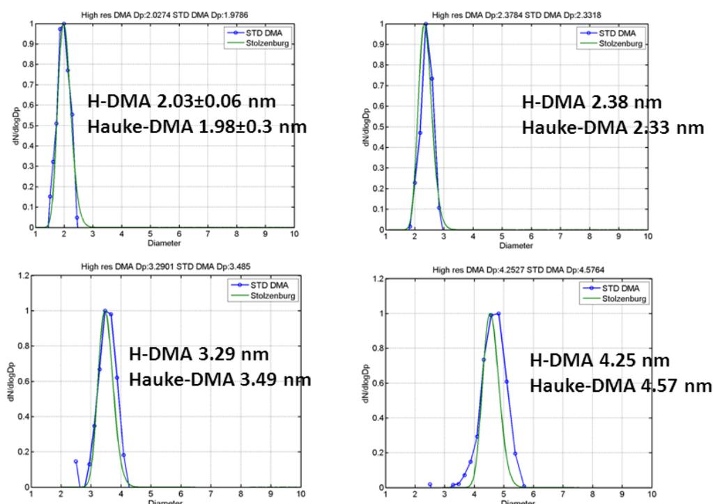
Figure 2. Calibration of the nano-MPSS (Hauke-DMA) against the high resolution H-DMA in nucleation mode range for four generated silver particle sizes (blue line measured and green theoretical size).
