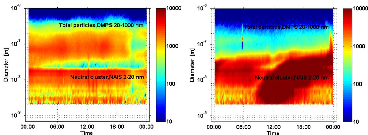
Figure 3. Merging MPSS and ion spectrometer spectras: Particle size distribution measured with the NAIS in 2–20 nm and with the MPSS in 20–1000 nm on April 4 (left) and April 19, 2011 in Hyttälä.
