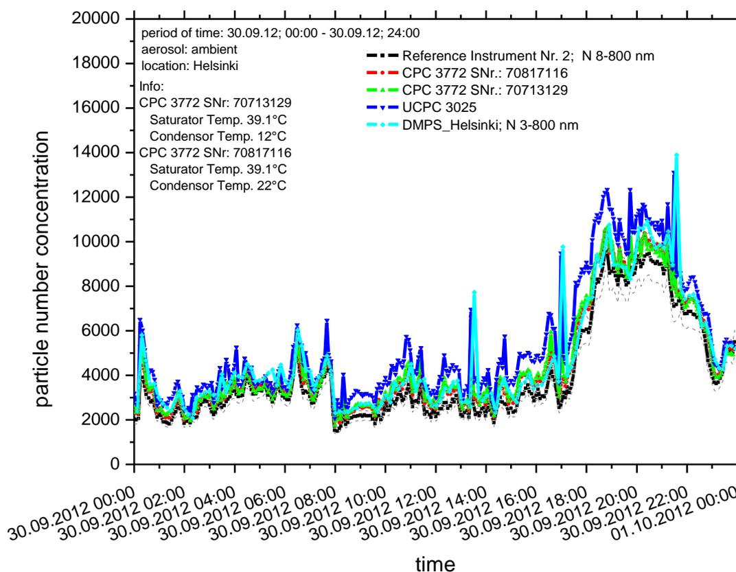
Figure 1. Total concentration comparison between nano-MPSS (DMPS-Helsinki), standard MPSS (Reference Instrument), several nano-Condensation Particle Counters (CPC 3025 and 3772's) when ambient sample was measured 24 hours on 30.9.2012 in Helsinki.
