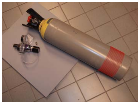
Picture 1) Round robin gas cylinder and pressure regulator with PFA tubing
