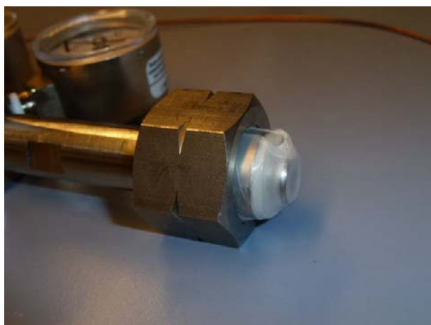
Picture 2) cylinder connector sealed with Parafilm tape.
