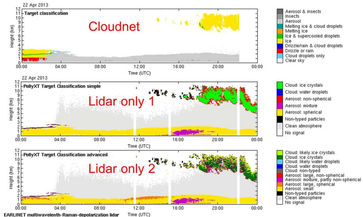
Fig. 6: Top: Cloudnet target classification (Hogan and O'Connor, 2004). Center and Bottom: Two different target classifications (following Fig. 5) as obtained from the multiwavelength-Raman-depolarization lidar PollyXT.
