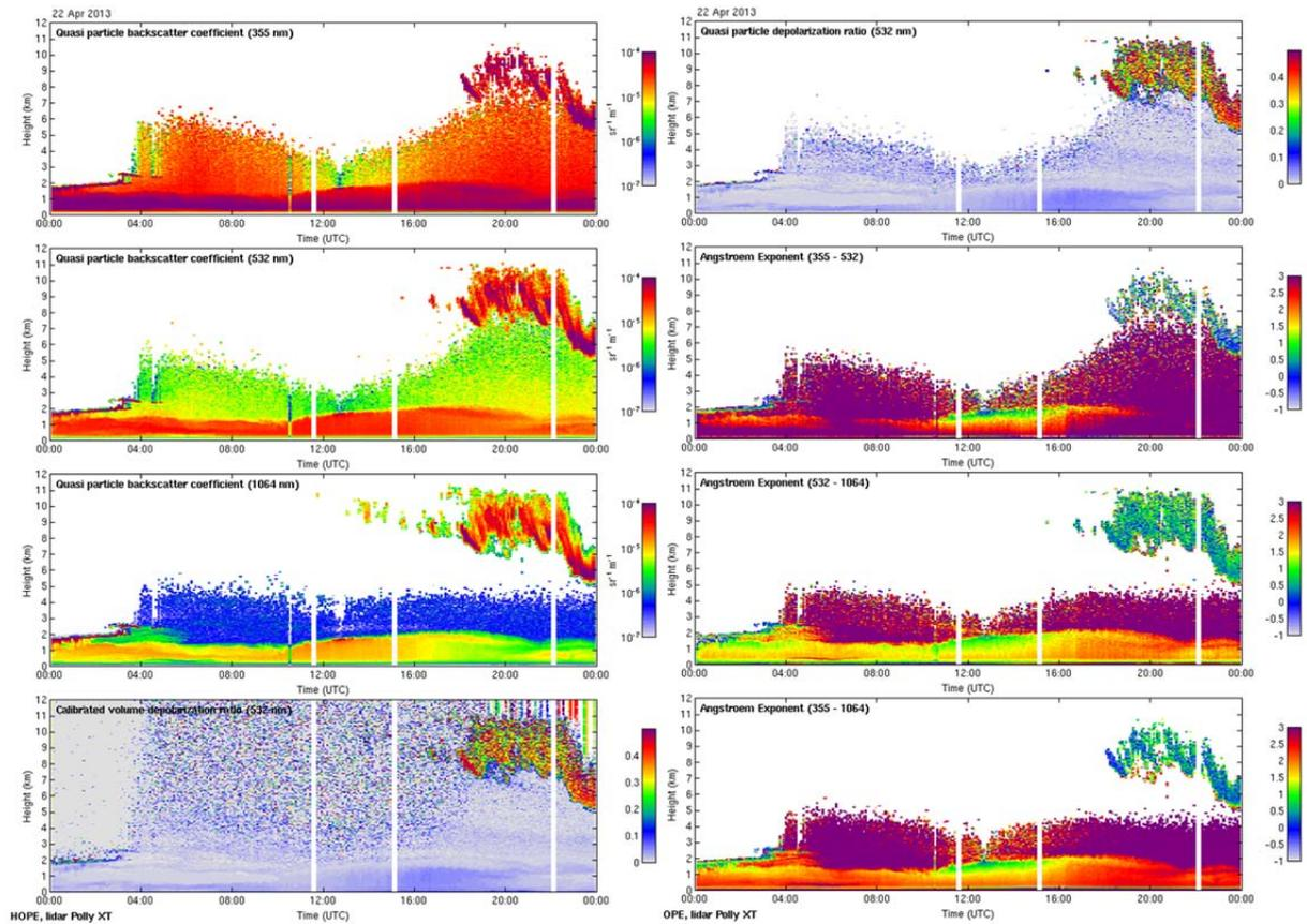
Fig. 3: Quantities obtained from the automatic lidar PollyXT in 24/7 mode. Left panels show the extensive properties and right panels the intensive properties. Three times a day the automatic depolarization calibration takes place indicated by the three white vertical bars.
