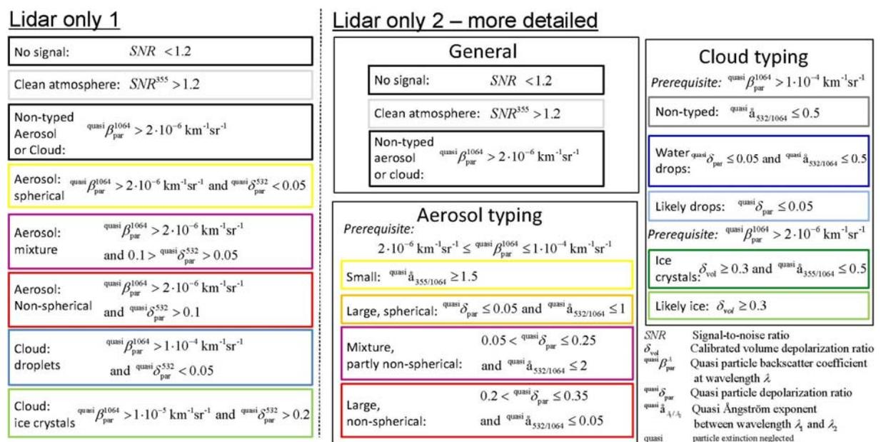
Fig. 5: Overview of classification scheme for aerosols and clouds as performed with the EARLINET lidar PollyXT. Two different schemes are presented.
