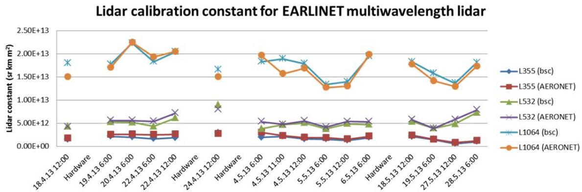
Fig. 2: Temporal evolution of the lidar calibration constant for 355, 532, and 1064 nm as obtained by two different methods (AERONET and backscatter=bsc) for the EARLINET lidar PollyXT.
