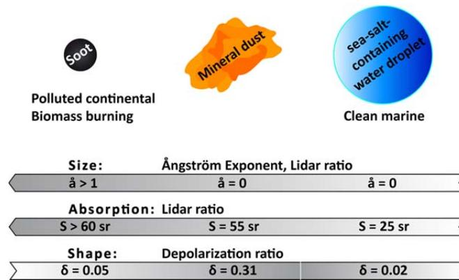
Fig. 4: Schematic illustration how different aerosol types could be classified by means of Ångström exponent, lidar ratio, and depolarization ratio (Tesche, 2011).
