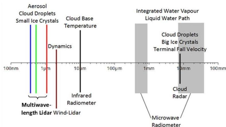
Fig. 1: Overview of wavelengths used by Cloudnet and EARLINET to characterize clouds, aerosols and meteorological parameters (Bühl, 2012). For the aerosol characterization, wavelengths in the visible range are best suited.
