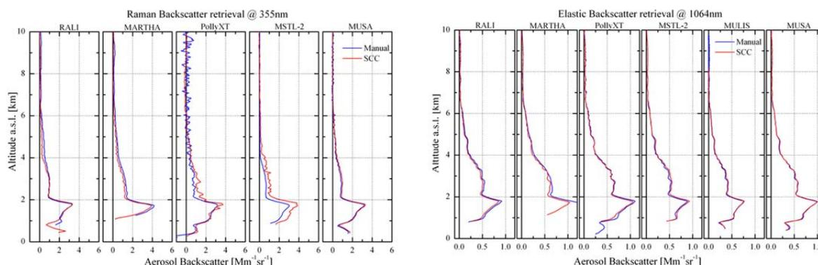
Fig. 7: Vertical profiles of backscatter coefficient at 355 and 1064 nm as obtained for five different lidar systems during EARLI09 in Leipzig. Blue lines show the manual analysis done by the operating group; red lines show the output of the Single Calculus Chain.
