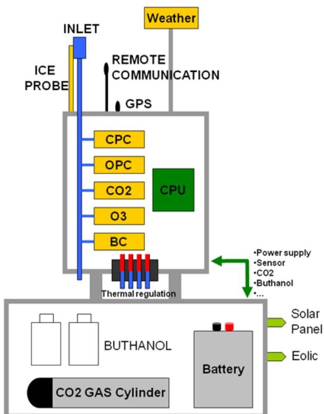
Figure 4: schematic description of the ACTRIS integrated station with the instrumented box containing all 5 instruments for gas and aerosol phases as well as the acquisition and communication systems. The second box contains batteries and standards / chemical for the instrumentation. A thermal regulation connects the 2 boxes.
