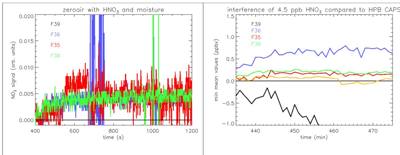
**Fig. 3 (left):** zoom of the HNO<sub>3</sub> region of the measurement, showing little response to the 5 ppbv HNO<sub>3</sub> provided in moist zero air. **Fig. 4 (right):** zoom of qualitative analysis of the interference of 4.5 ppb HNO<sub>3</sub> in dry zero air, based on a fit from NO<sub>2</sub>-sonde data to HPB CAPS data.
