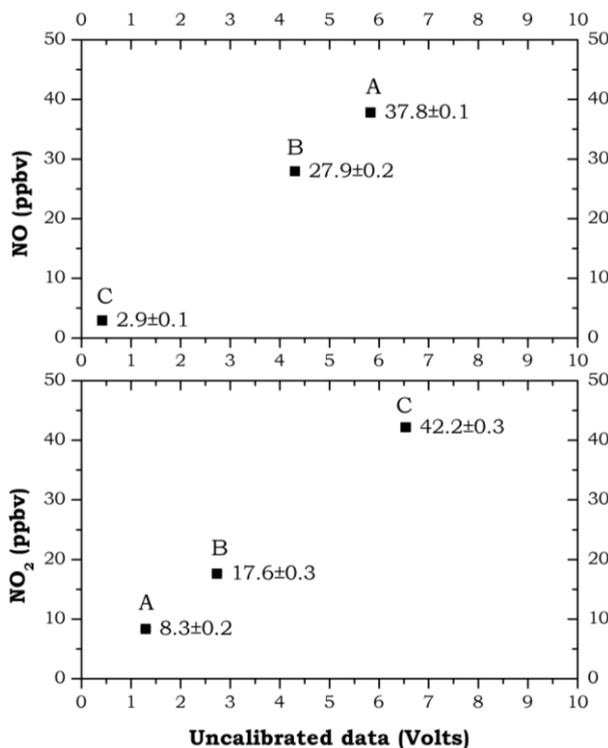
**Figure 4:** Identification of the unknown NO and  $\text{NO}_2$  concentrations (in ppbv) of 3 different gas mixtures.
