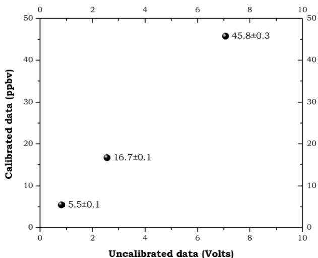
Figure 3: Identification of the NO concentration of 3 unknown samples (in ppbv)
