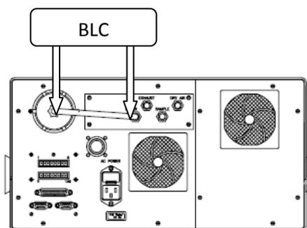
Figure 1 (Rear panel of the thermo 42C instrument used): The BLC has been connected in between the filter and the sample and it was turned on and off with the use of a chrono-plug timer.
