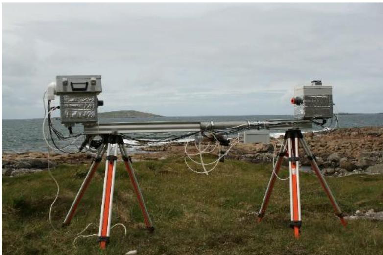
*Fig 2 Set-up of the new CE-DOAS instrument at the Mace Head research station for observations of IO.*
