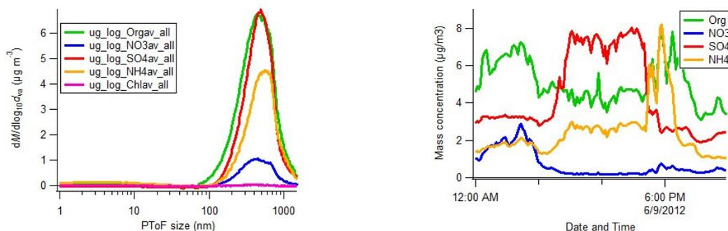
Figure 5. Size distribution and mass concentration of aerosol's components at ground on June 9
