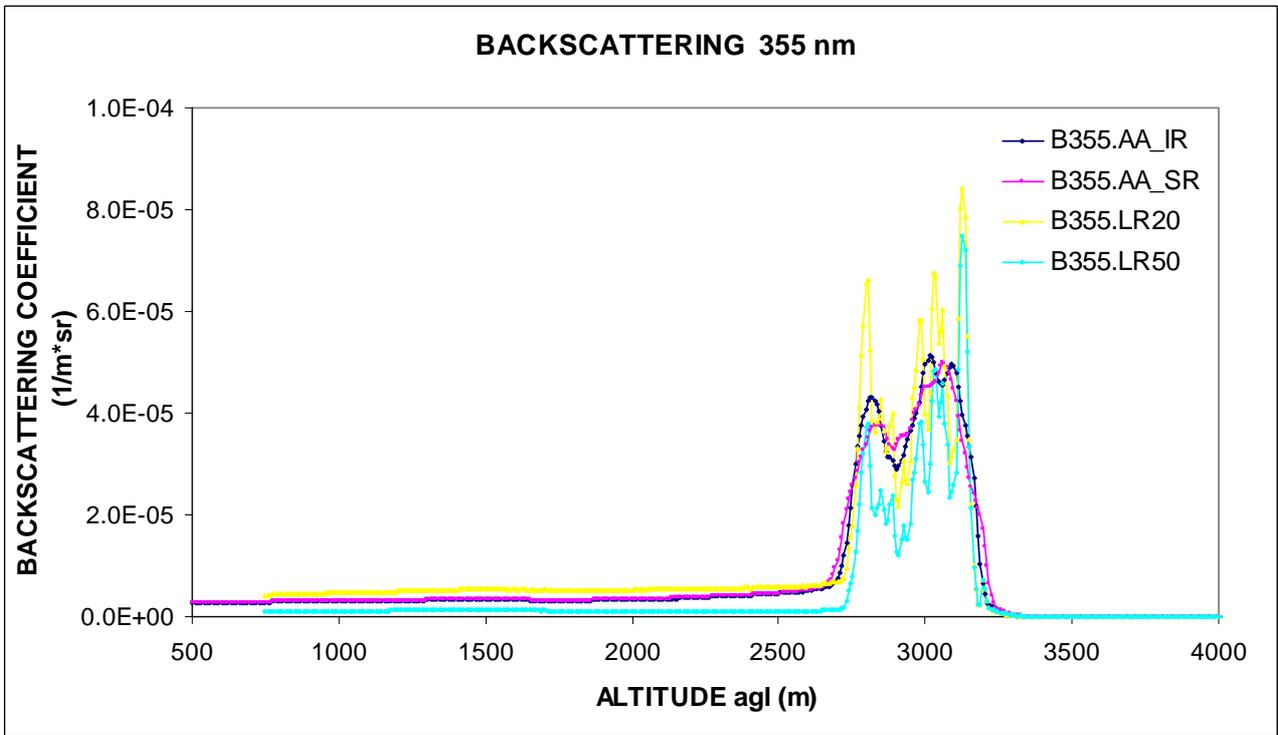
Figure 8. Profiles of the backscattering coefficient at 355 nm by the Klett-Fernald (assuming lidar ratio values of 20 and 50) and the Ansmann algorithm ((SR) same resolution function for backscattering and extinction. (IR) Different resolution function for backscattering and extinction).
