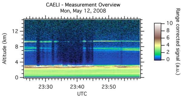
Fig. 4. Far range corrected signal at 1064 nm.
