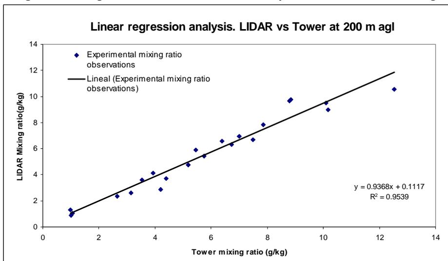
Figure 3. Linear regression analysis between lidar and tower mixing ratio observations at 200 m agl.
