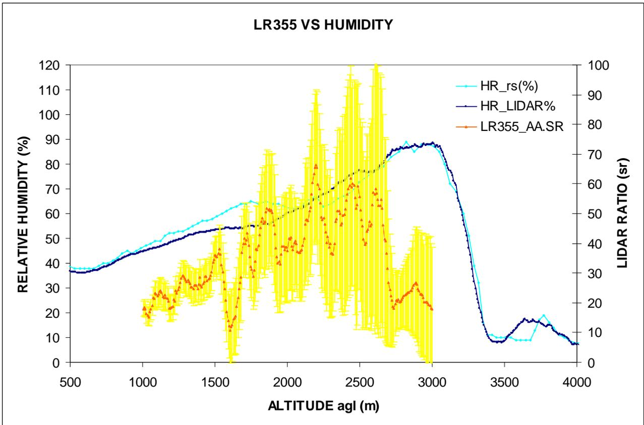
Figure 7. Profiles of the lidar ratio at 355 nm (SR same resolution function for backscattering and extinction) and relative humidity estimated by lidar and radiosounding.
