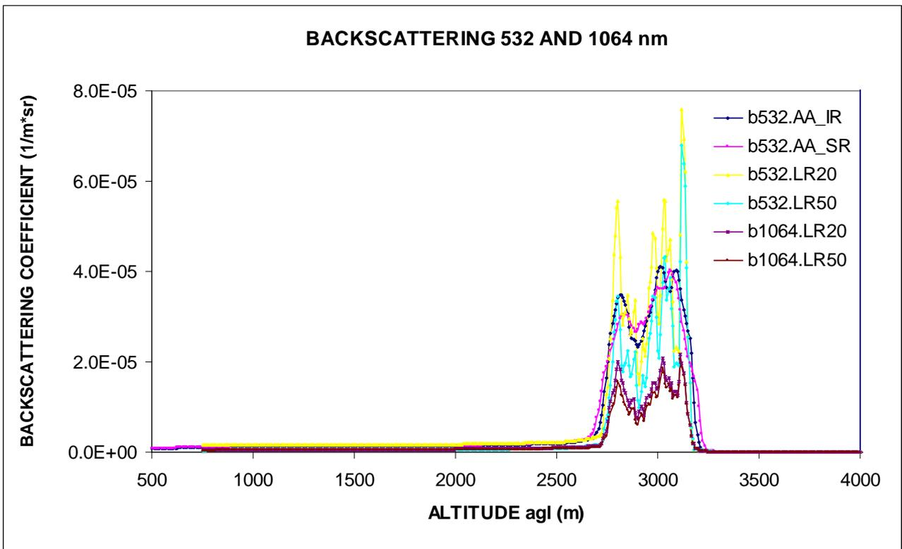
Figure 9. Profiles of the backscattering coefficient at 532 and 1064 nm by the Klett-Fernald (assuming lidar ratio values of 20 and 50) and backscattering coefficient at 532 nm by the Ansmann algorithm ((SR) same resolution function for backscattering and extinction. (IR) Different resolution function for backscattering and extinction).
