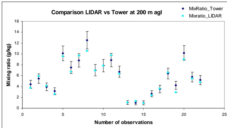
Figure 2. Mixing ratio measurements obtained by lidar and tower at 200 m agl.
