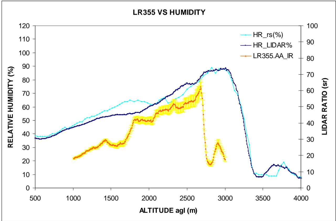
Figure 6. Profiles of lidar ratio at 355 nm ((IR) Different resolution function for backscattering and extinction) and relative humidity estimated by lidar and radiosounding.
