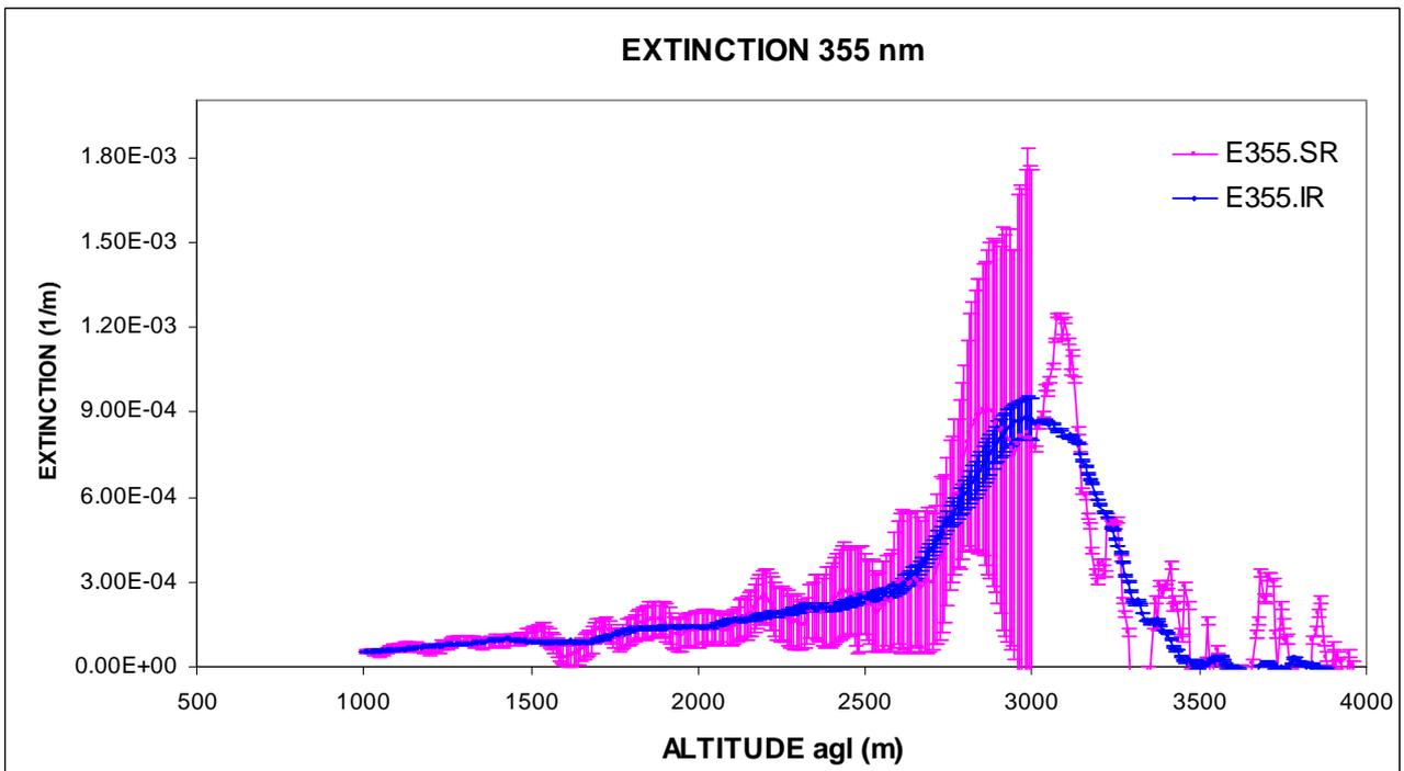
Figure 8. Profiles of the extinction coefficient at 355 nm (IR=Resolution function of 300, SR = Resolution function of 150) and its errors.
