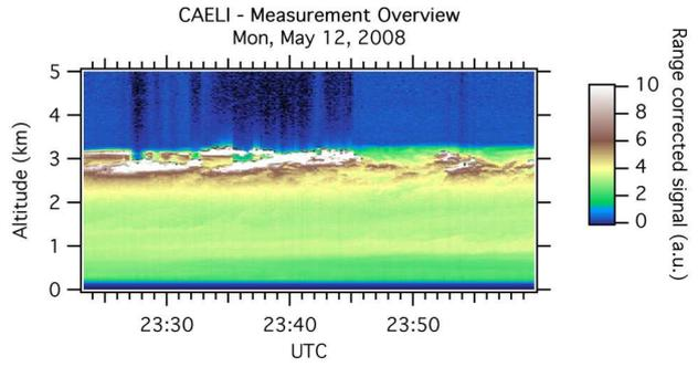
Fig. 5. Near range corrected signal at 1064 nm.
