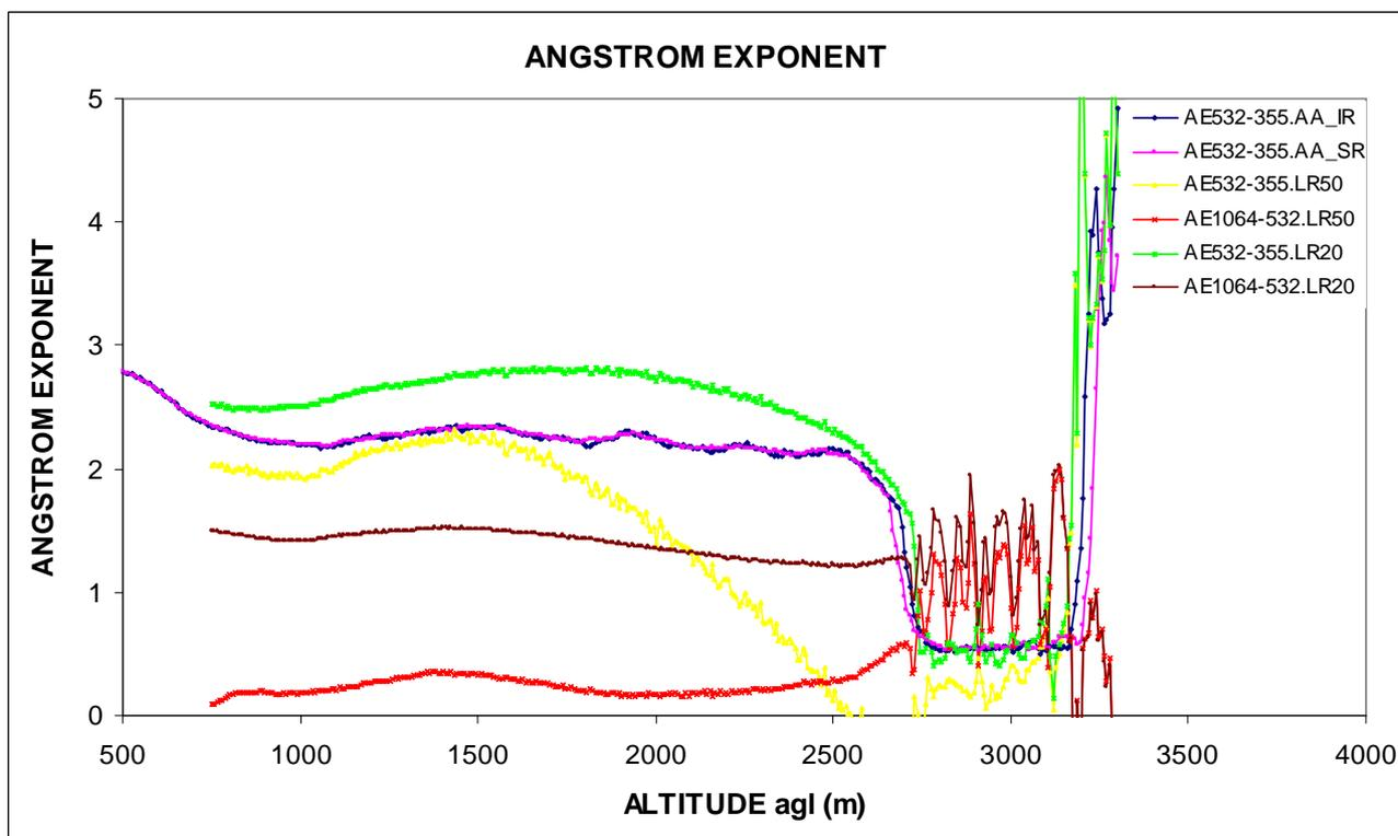
Figure 10. Profiles of the backscatter-derived angström exponents from previous backscattering coefficient retrievals.
