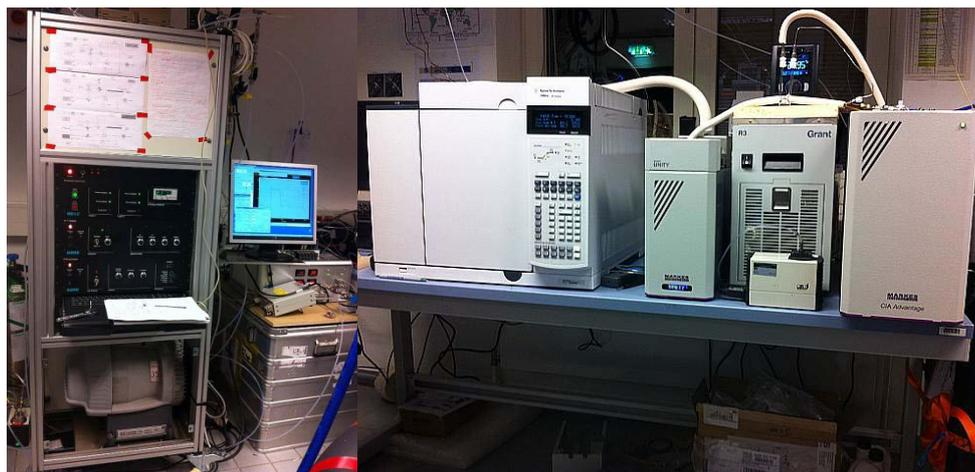
Figure 1 : PTR-ToFMS (left) and TD/GC/FID-MS (right) instruments deployed by Mines Douai in the guest lab
