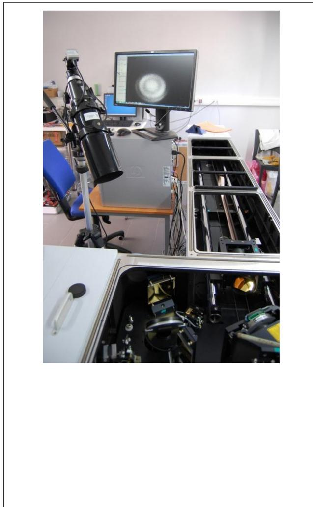
*Illustration 1: A telescope is mounted on a tripod outside the FTIR spectrometer, such as to observe monochromatic light (laser light that has passed through a diffuser) after it has passed the interferometer, giving rise to Haidinger fringes that are visible on the computer image.*
