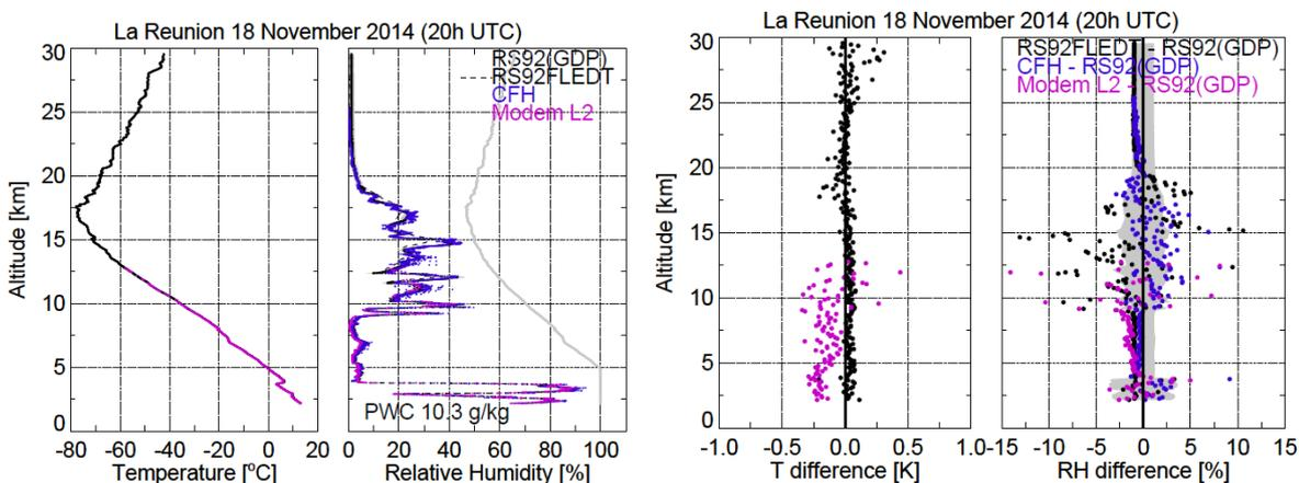
Figure 1: Radiosounding at Maïdo observatory on November 18, 2014 during the Pre-MORGANE experiment (ACTRIS TNA: MAIDO-3 WV-PROFILES-MAIDO project). Left: Temperature (°C) and relative humidity (%RH). Right: as for left but for differences between sondes or data processing methods. Employed radiosondes are MODEM M10, Vaisala RS92 and CFH.
