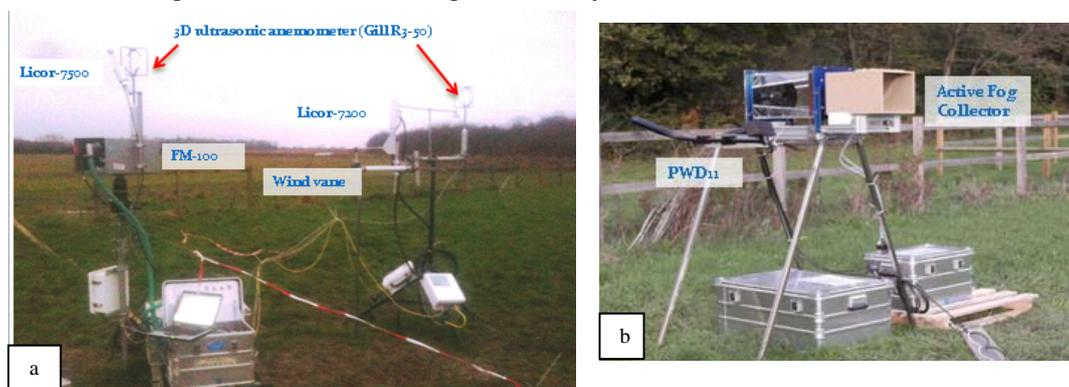
Figure 1. The two eddy covariance measurement setups (left) and the active fog collector (right) at the SIRTA site
